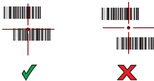
Figure 46 RS6000 Pick List Mode with Multiple Barcodes in Aiming Pattern
