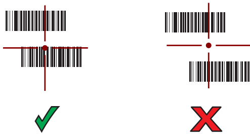
Figure 43 RS507/RS507X Pick List Mode with Multiple Barcodes in Aiming Pattern
