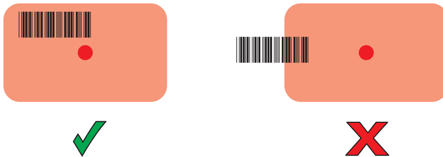
Figure 49 DS3608/DS3678 Pick List Mode with Multiple Barcodes in Aiming Pattern
