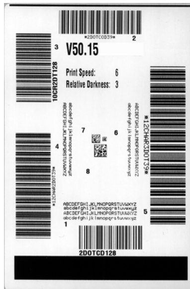
Figure 19 • Sample Darkness and Speed Test Label
