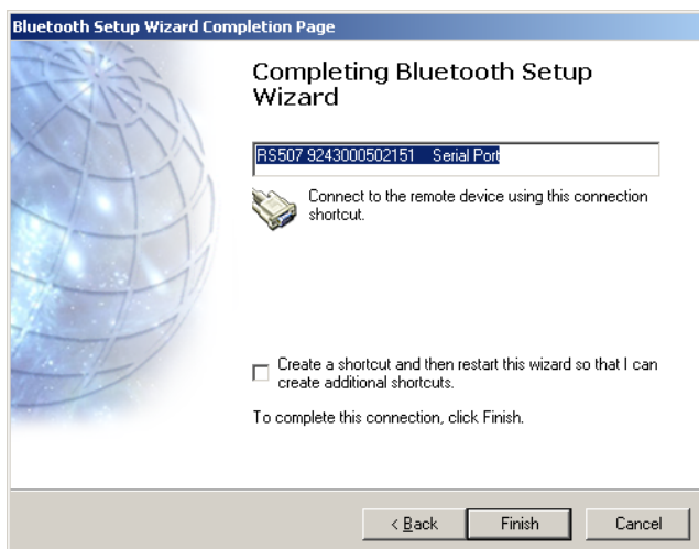
Figure 7-43 Bluetooth Setup Wizard - SPP connection with RS507 as a Slave
