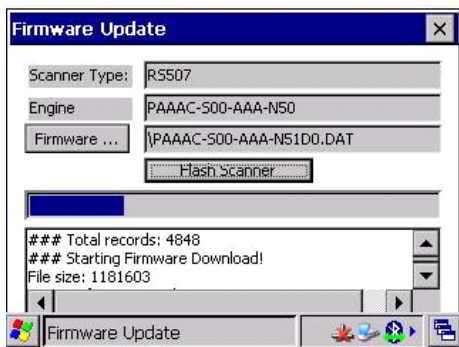
Figure 4-26 Firmware Update Screen - "Starting Firmware Download!" Message
