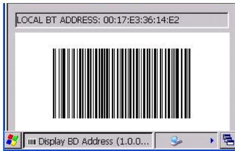
Figure 1-12 Pairing Bar Code Example as Shown on the Mobile Computer Screen
