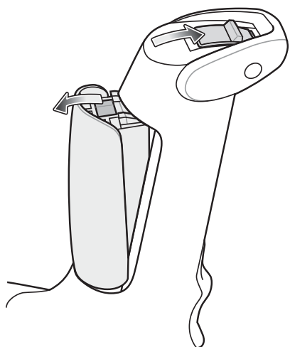
Figure 1-4 RFID Sled Battery Removal
