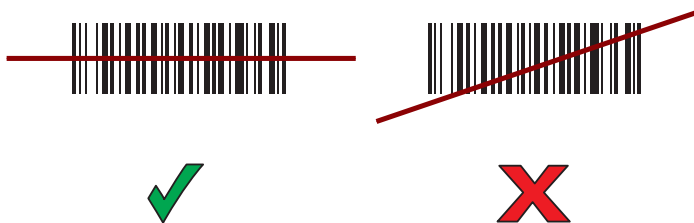
Figure 38: Linear Scanner Aiming Pattern
