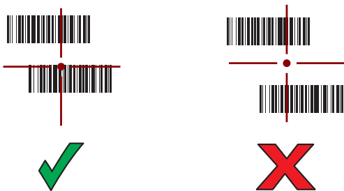
Figure 34: Pick List Mode with Multiple Bar Codes in Aiming Pattern
