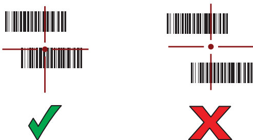
Figure 39: Pick List Mode with Multiple Bar Codes in Aiming Pattern
