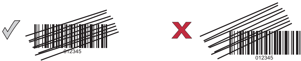
Figure 2-3 Acceptable and Incorrect Multi-Line Aiming
